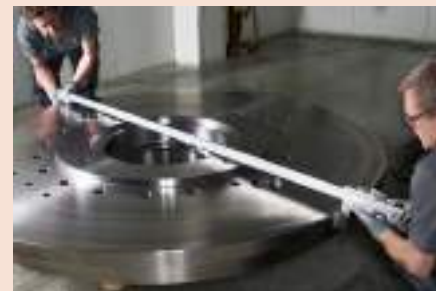
Radiused jaws for accurate ID measurement
